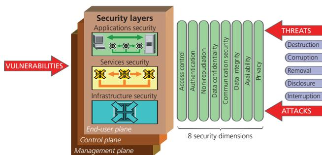
This figure depicts the concept of protecting a network by security dimensions at each security plane of each security layer in order to provide a comprehensive security solution. It should be noted that, depending on a given network's security requirements, it might not be necessary to have all architectural elements implemented or to have a complete set of the security dimensions, security layers and security planes.
